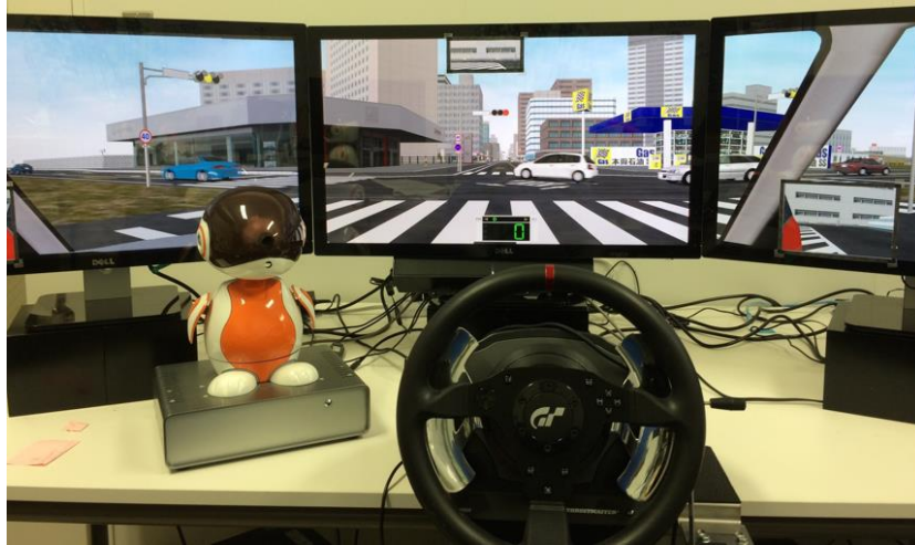
Figure 1: Overview of the Driving Simulator System (The depth, width, and height of the robot are 21, 26, and 34 cm, respectively. The degrees of freedom of the head, arms, and body are 3, 1, and 1.)
